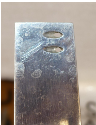
Photo shows an MHZ rudder where the water can enter the rudder from both sides. © GNP
