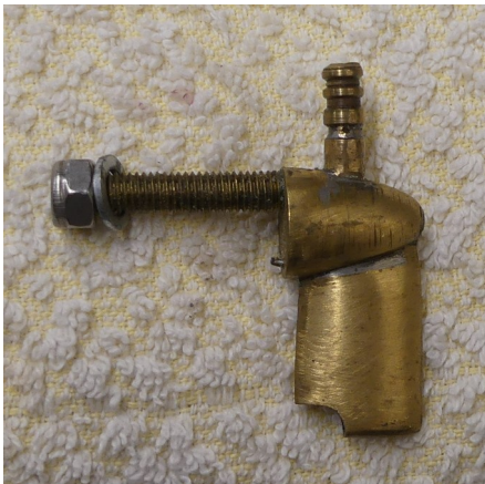
Photo shows a water pick up designed to be bolted through the transom – water is collected via a hole in the base of the downward pointing shaped strut and a water connection is made from the nipple through the transom. © GNP
