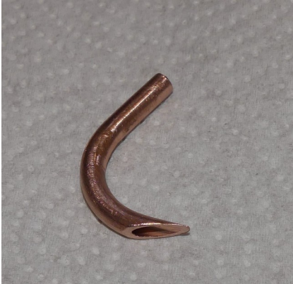
Photo of a copper pipe based water pick up. © GNP
