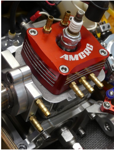
Photo shows a 3-in 2-out water arrangement on a Zenoah 320. © GNP
